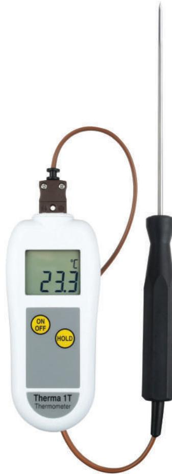
**INSTRUMENT OPERATION** - Where applicable, connect a probe via the socket located at the top of the instrument. Switch the instrument on and apply the tip of the probe to the substance or medium to be measured. The instrument reading may take a few seconds to stabilise, depending on the nature of the measurement and sensitivity of the probe.
